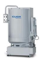
The Cuda 2840 is the next step up in the compact Front-Load Automatic Parts Washer Models. The 2840 features a turntable diameter of 28-inches, working height of 40-inches, and load capacity of 1000 lbs. The 2840 Series is equipped with a 3 HP vertical seal-less pump producing 50 GPM at 45 PSI.
